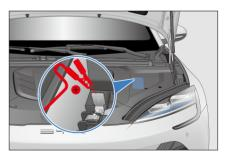
4. Connect the other end of the red positive (+) cable to the positive (+) terminal of the charged low voltage distribution box of the rescue vehicle.
