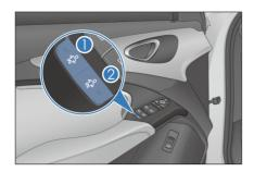
To activate child protection locks, press the child protection lock button ① or ②. The corresponding indicator lights up. At this time, the occupants cannot open the rear door on the corresponding side. To unlock the door, press the child protection lock button for the corresponding side again or use the exterior door handle.
