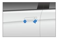
2. Once the right side is extended, pull the middle of the handle outward to extend the handle.
