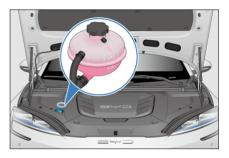
Refill coolant to the MAX line if the level is below the MIN line. Check the cooling system for leakage.
