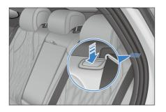
2. There is an emergency unlocking mechanism on the lid cover, open the lid cover in the vehicle by pulling the emergency opening lever on the left (as shown in the figure).
