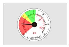
If the tire pressure reaches between 180 and 320 kPa (green and yellow areas shown in the figure), remove the kit as soon as possible and drive at a speed below 80 km/h within one minute, with the furthest driving distance not exceeding 10 km, so that the tire sealant is evenly distributed within the tire.
