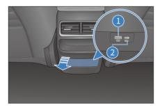
The power outlet can be used only when the ignition is on.
