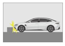
The vehicle's nose hits the ground when going down a steep slope.
