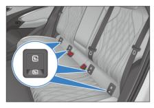
• Anchor supports (for the top tether) are provided at the rear outboard seat.
