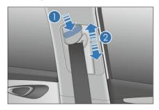
5. Pull the shoulder belt firmly to check that the adjuster is locked.
