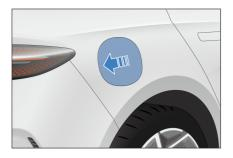
Open the vehicle charge port cap, and make sure that no obstacles exist between the head of the charging connector and the end of the charging socket.
