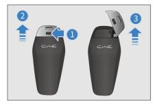
After using the mechanical key, insert it in the opposite direction and close the back cover of the smart key.
