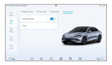
When enabled, the system raises an alarm if obstacles are found around the vehicle: when disabled, it does not.
