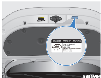
Battery Position Indication Label
