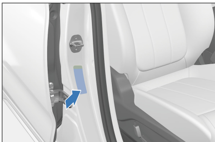
Side airbag labels are attached on the lower part of the left and right B-pillars.
