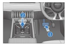
· When the "OK" indicator lights up on the cluster, the vehicle is powered on.
