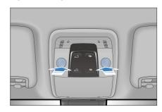
· Press the interior light buttons to turn on left/right interior lights. Press again to turn them off.
