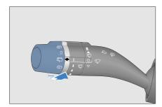
position and released, the wiper will operate once or twice further after the spray has stopped.
