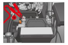
3. Connect the other end of the red positive (+) cable to the positive terminal (+) of the charged battery of the rescue vehicle.
