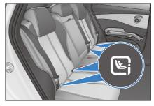
Rear outboard seats are equipped with tether strap anchorages on the back.
