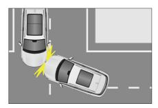
The vehicle hits a columnar object on one side
