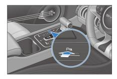
There will be an alarm if obstacles are found surrounding the vehicle when the system is powered on. There will be no alarm when the vehicle is powered off.
