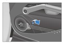
• When the trunk lid is open and the switch is pulled for more than a second, the lid closes automatically. The lid stops closing after the switch is released.
