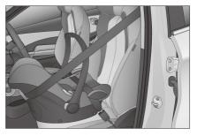
The rear outboard seats are equipped with ISOFIX/i-Size anchorages\*. The anchorage locations are identified by a marking (see the figure) located on the seat back, directly above the associated anchorages.
