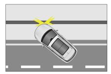
Parts other than the passenger compartment receive side impacts.
