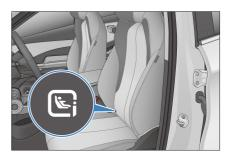
The front passenger seat is equipped with a tether strap anchorage\* on the back
