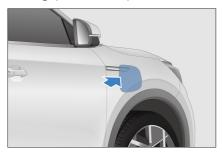
Open the hatch and remove the charge port cap. Make sure the port is not obstructed in any way.
