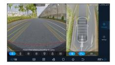
· After the vehicle starts, the image before last power-off will be displayed on the invisible panoramic screen. Foreign bodies in the underbody and surrounding blind areas may be inconsistent with the actual ones. The underbody image will be updated in real time only after the vehicle has moved, which must be driven beyond its length for a complete update.
