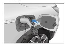
After the connection is made. discharge begins and respective information is displayed on the instrument cluster
