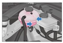
If the level is below the MIN line, refrigerant should be refilled to the MAX line. Check the cooling system for leakage.
