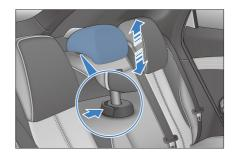
4. Installing the head support: insert the head support poles into the bushing with the grooves facing forward. Press the head support adjustment button, press the head support down to a proper position, and release this button.
