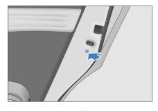
The usage tip sticker of the charging connector is attached to the inner surface of the charging port cover.
