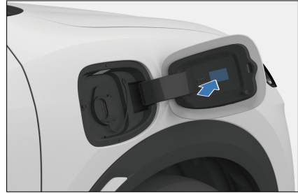
The charging warning label is attached on the inside of the charge port door.
