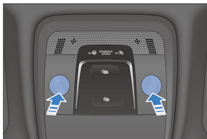
Front interior lights (Configuration 1)
