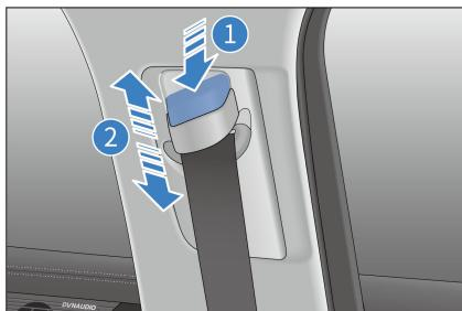
5. Pull the belt firmly to check that the adjuster is locked.
