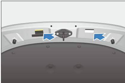
The charging warning label and the charge port label are attached on the inner side of the charge port door.
