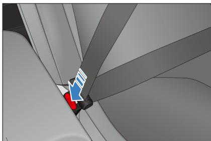
4. Adjust the height of the (front) seat belts for optimum comfort and protection.
