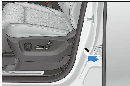
The representative information label is attached at the lower sheet metal sink of the left B-pillar.
