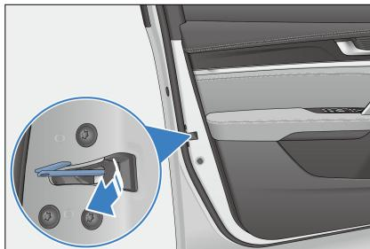
3. Open the driver's door after locking other doors. Lift and hold the driver's door handle and pull it to its maximum angle.
