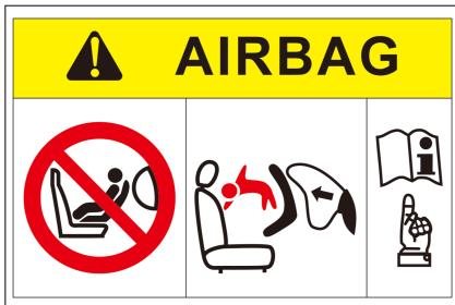
**Always follow the instructions below when using a child restraint on the front passenger seat:**
